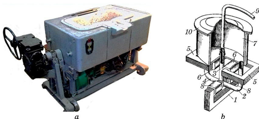
Fig. 1. External view ( a ) and general scheme ( b ) of the magnetohydrodynamic installation MDI-6A: 1—crucible; 2, 3, 4—branches of the induction channel; 5—closed magnetic cores of the inductors; 6—inductor coils; 7—open magnetic core of the electromagnet; 8—electromagnet coils; 9—detachable metal duct; 10—crucible cover.
